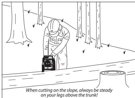
When cutting on the slope, stay as shown in the Figure. To have a full control over the chainsaw at the moment of full cross-cut, reduce the pressure in the final cut phase, still holding chainsaw handles firmly in your hands. **Attention, the chain may not touch the ground!** When
