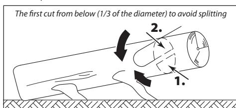
If the trunk lies on the ground by its one end, see Figure, cut at first 1/3 of trunk diameter from the bottom side and then the remaining part from the top as deep as the bottom cut.
