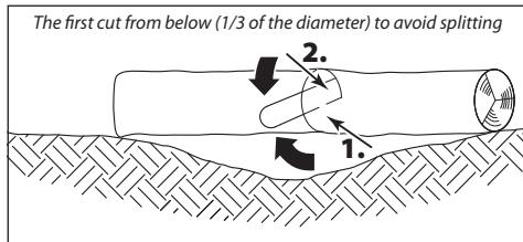
If the trunk lies above a field depression supported on its ends, see Figure, cut at first 1/3 of trunk diameter from the bottom side and then the remaining part from the top as deep as the bottom cut.
