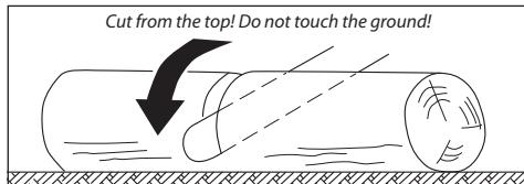
If the whole trunk length is supported uniformly, see the Figure, cut from the top.
