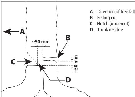
Cut a notch at the right angle to the tree as deep as 1/3 of tree diameter. To make the notch, the horizontal cut shall be done at first to avoid jamming (seizing) of the chainsaw or the guide bar when starting the second oblique cut of the notch.
